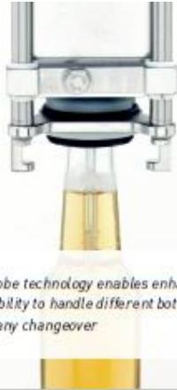
*Level probe technology enables enhanced accuracy and flexibility to handle different bottle sizes without any changeover*
